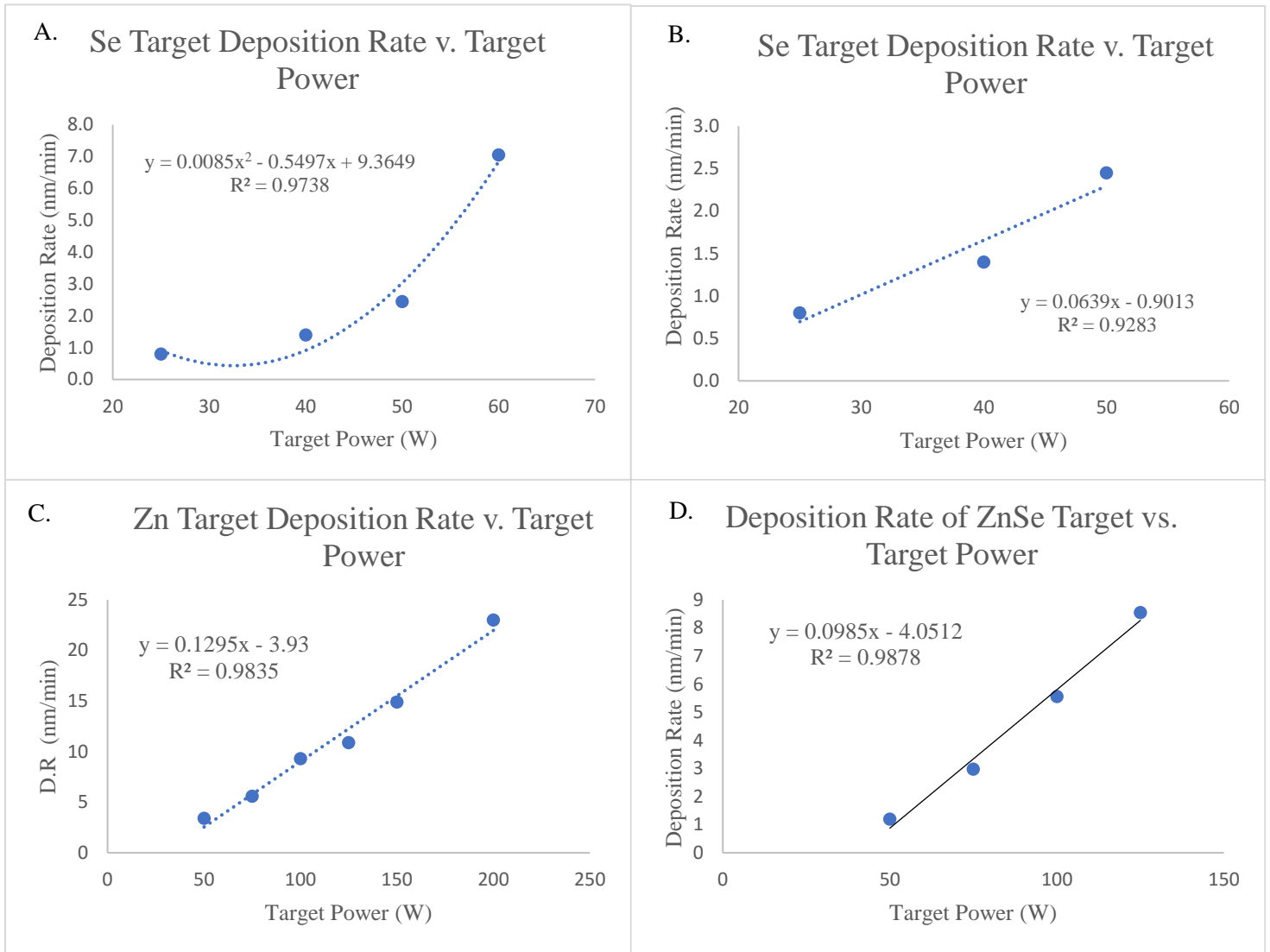
Figure 3: Deposition rate vs power for A) the Se target with nonlinear fit, B) the Se target subset, with linear fit, C) the Zn target with linear fit, and D) the ZnSe target, with linear fit.
