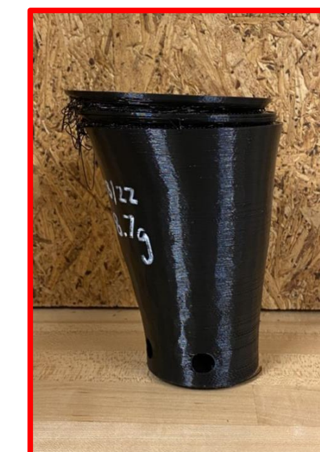
Poor quality socket with shifted layers
