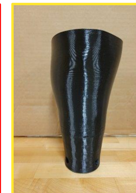
Poor surface finish
