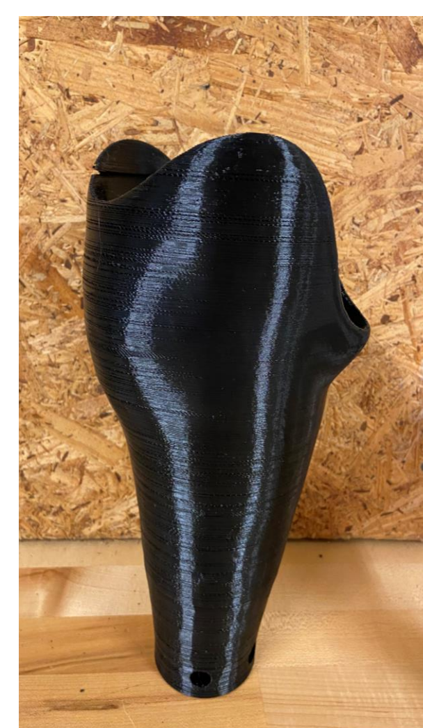
3D Printed Transtibial Socket
