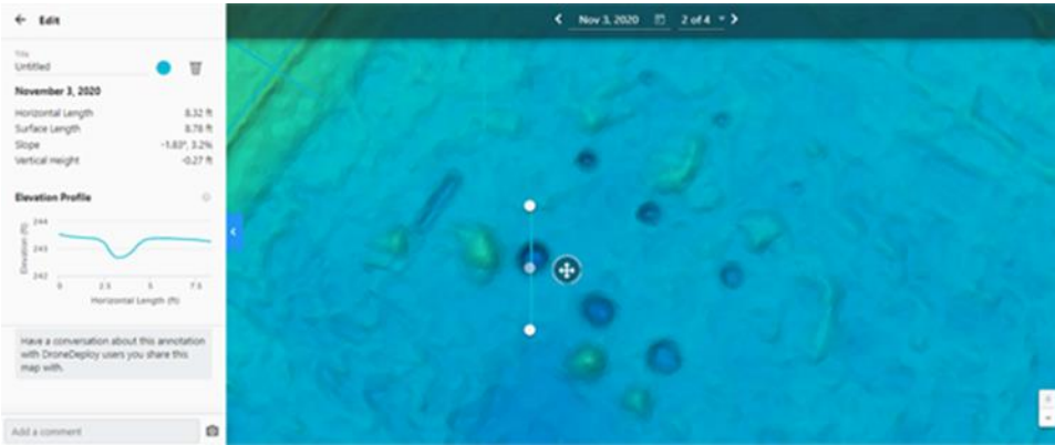
Figure 7- Shows an example of measuring holes using DroneDeploy (Should be Figure 7)
